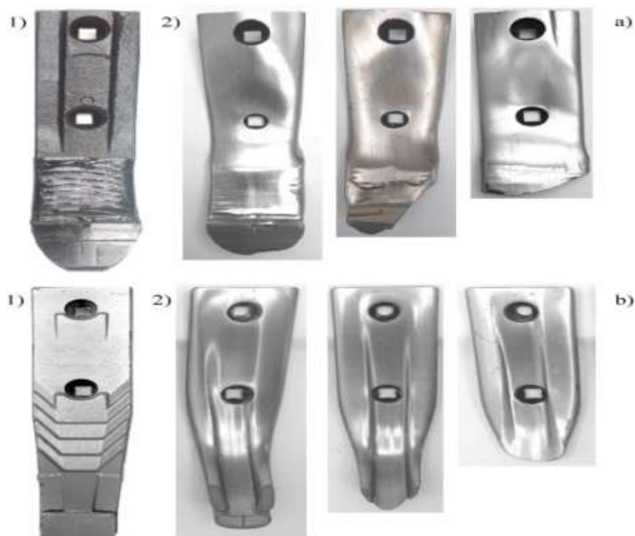
Fig. 9. Exemplary stages of wear of the coulters: a) A/1; b) B (1 - new element, 2 - elements after operation in soil).
